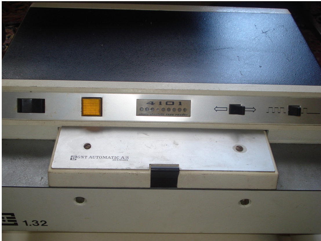
Tape reader controls; L-R, Power switch, Power indicator, the bit pattern display, direction switch and continuous/single step switch.
