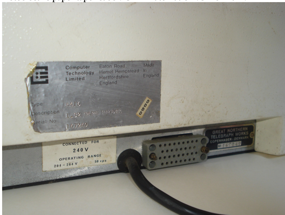
CTL Badge label, power cable entry, data connector to the Modular One and the manufacturers label "Great Northern Telegraph Works Copenhagen Denmark". The serial number is 147249.
